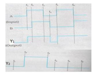
Identify the 'equivalent gate' needed in each case. Show how one can connect an appropriate number of (i) NAND (ii) NOR gates respectively in the two cases to get these 'equivalent gates'.
